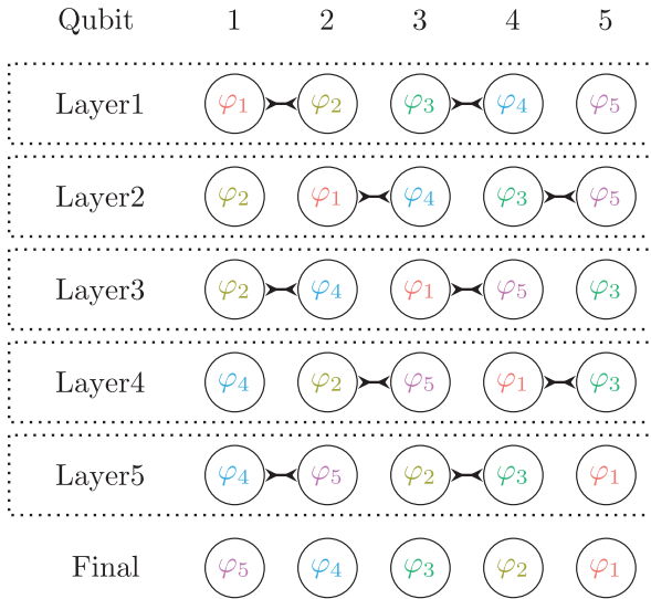
FIG. 1. A depiction of how the canonical Jordan-Wigner ordering changes throughout five layers of fermionic swap gates. Each circle represents a qubit in a linear array (qubits do not move) and \varphi_p labels which spin-orbital occupancy is encoded by the qubit during a particular gate layer. The lines in between qubits indicate fermionic swap gates which change the canonical ordering so that the spin orbitals are represented by different qubits in the subsequent layer. After N layers, the canonical ordering is reversed, and each spin orbital has been adjacent to all others exactly once.
