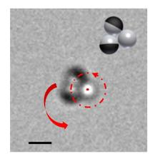
**SI Figure 5.** Motor/non-motor interaction: rotational motion with the non-motor anchored to the glass surface (taken from SI Video 7). Scale bar, 2 µm. Conditions, as in Figure 1.
