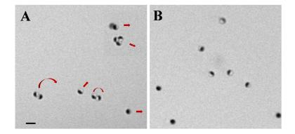
**SI Figure 1.** Control experiments (taken from SI Video 3): Janus micromotors with (A) and without (B) hydrophobic coating. The latter offers simultaneous movement of single, doublet, and triplet motor assemblies. Scale bar,  $2 \mu m$ . Conditions, as in Figure 1.
