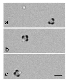
**SI Figure 3.** 'On-the-fly' capture of a non-motor particle by a triplet micromotor assembly. Time-lapse images of a, b, and c have been taken from SI Video 6 in 1 second intervals. Scale bar, 3 µm. Conditions, 5% hydrogen peroxide.
