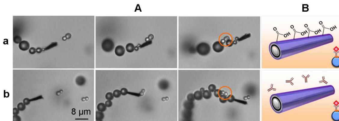
**SI Figure S-3.** Interaction between nanomotors and AntiIgG-IgG-modified S-PP, navigating in a glass slide (A). Negative controls: PEDOT/PEDOT-COOH (a) and PEDOT-anti-IgG-incubated nanomotors (b), respectively. Corresponding sketches for a) and b) and modified S-PP (B), respectively. Contacted but unloaded particles, highlighted by an orange circle.
