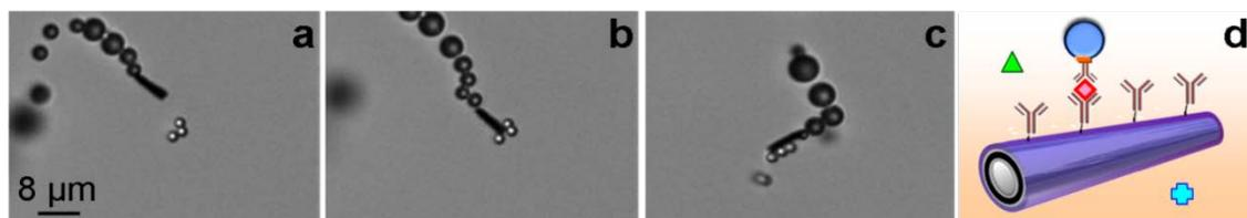
**SI Figure S-4.** Anti-IgG-functionalized-microtransporters displaying an immediate ‘on the fly’ protein capture upon contacting the tagged-IgG target being present in a concentration of 20 µg/ml in the presence of a 10-fold excess of BSA and lysozyme proteins (Experiments performed on a glass slide). IgG, BSA and lysozyme, red rhombus, green triangle and blue cross, respectively.
