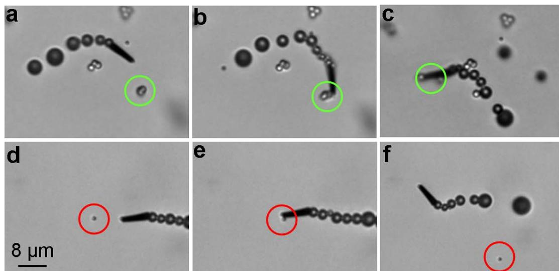
**SI Figure S-2.** Modified microengine capturing and transporting a IgG-anti-IgG-modified-PP complex (delineated by green circles), and interacting (but not loading) with PP of smaller size (delineated by red circles).
