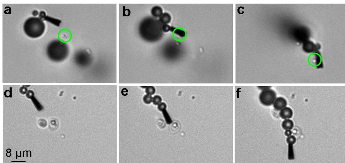
**SI Figure S-5.** Selective binding and transport of the small rod-shaped (~2 µm length) *S. aureus* bacteria (delineated by green dotted circles) vs the bigger round-shaped *S. cerevisiae* cells (unlabeled, ~5 µm in diameter), unloaded even when after multiple contacts with the antiproteinA-modified microtransporter.
