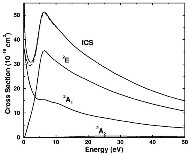
FIG. 1. Integral cross section for elastic scattering of electrons by  $\text{CH}_3\text{SiH}_3$ , along with its  $C_{3v}$  symmetry components. Below 10 eV, the integral cross section is shown both with (solid line) and without (dashed line) a correction for long-range scattering.
