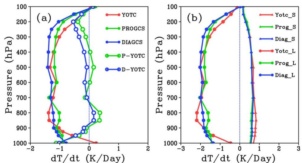
**Figure 9.** Vertical profiles of global mean radiative heating rate (unit:  $K d^{-1}$ ) from (red line) YOTC and model simulations with (green line) PROGCS and (blue line) DIAGCS during 00UTC, 2 July and 00UTC, 3 July 2009. In Figure 9a, it shows (closed circle) the total (LW + SW) radiative heating rate and (open circle) its differences compared with YOTC and it plots the heating rates from (closed circle) LW and (closed triangle) SW in Figure 9b, respectively.
