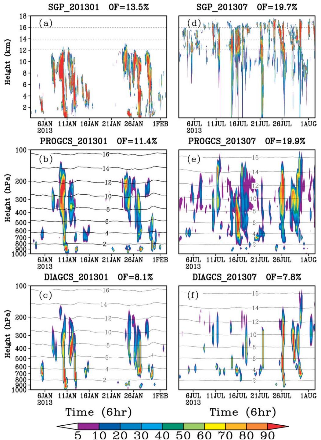
**Figure 3.** Six-hourly vertical distributions of cloud cover (a, d) from ARM observations, and simulated with (b, e) PROGCS and (c, f) DIAGCS over SGP site for (left column) January and (right column) July 2013 (unit: %). The shaded areas indicate the cloud cover greater than 5% and the contour lines represent the height (unit: km). The value at the top-right of each graph is the occurrence frequency of cloud cover.
