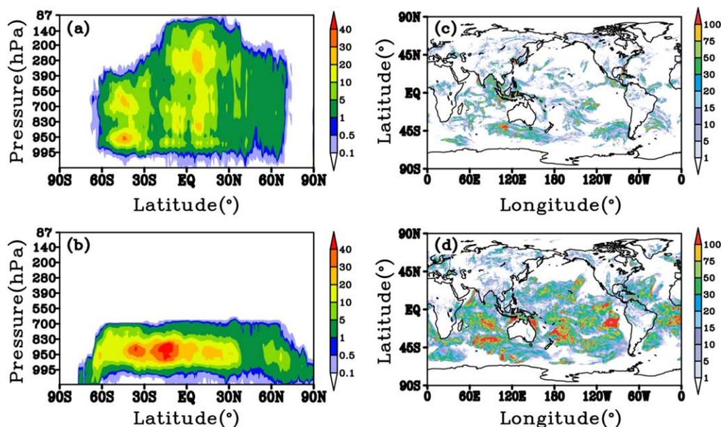
**Figure 1.** (left column) Zonal-mean cross sections and (right column) global distributions at 850 hPa of cloud-cover formation rate from (a, c) deep convection and (b, d) shallow convection processes averaged from 1 to 3 July 2013 (unit: %/DT).
