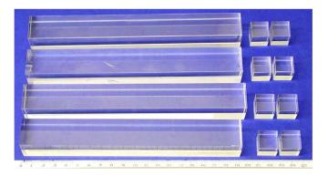
Fig. 2. A photo showing four long ( $2.5 \times 2.5 \times 20$  cm) crystal samples, from top to bottom: SIC BGO, CPI LYSO, SG LYSO and CTI LSO, together with two corresponding small cubic samples ( $1.5 X_0$  cube) from each manufacturer.
