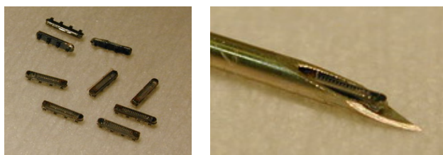
Figure 7. Microfabricated needle-implantable parylene-based IOP sensors: (left) released devices; (right) a fabricated device situated inside a 19-gauge hypodermic needle.
