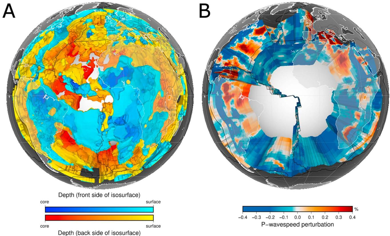
**Figure 4.** MIT-P08 tomographic model (Li et al., 2008) overlain with coastlines in white and tectonic plate boundaries in black. The gray interior of the continents is semitransparent. (a) A seismic velocity anomaly isosurface colored by depth. (b) Vertically extruded cross sections are shown along tectonic plate boundaries.
