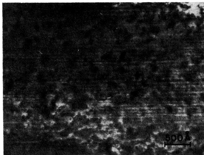
Figure 2: Dark field transmission electron micrograph showing the cross section of AlGaAs grown on the side facet of a groove, using the (200) reflection. The quasi-periodic contrast corresponds to an OSE superlattice (see text), with a period of  $70 \text{ \AA}$ . The [111] direction is vertical in the micrograph.
