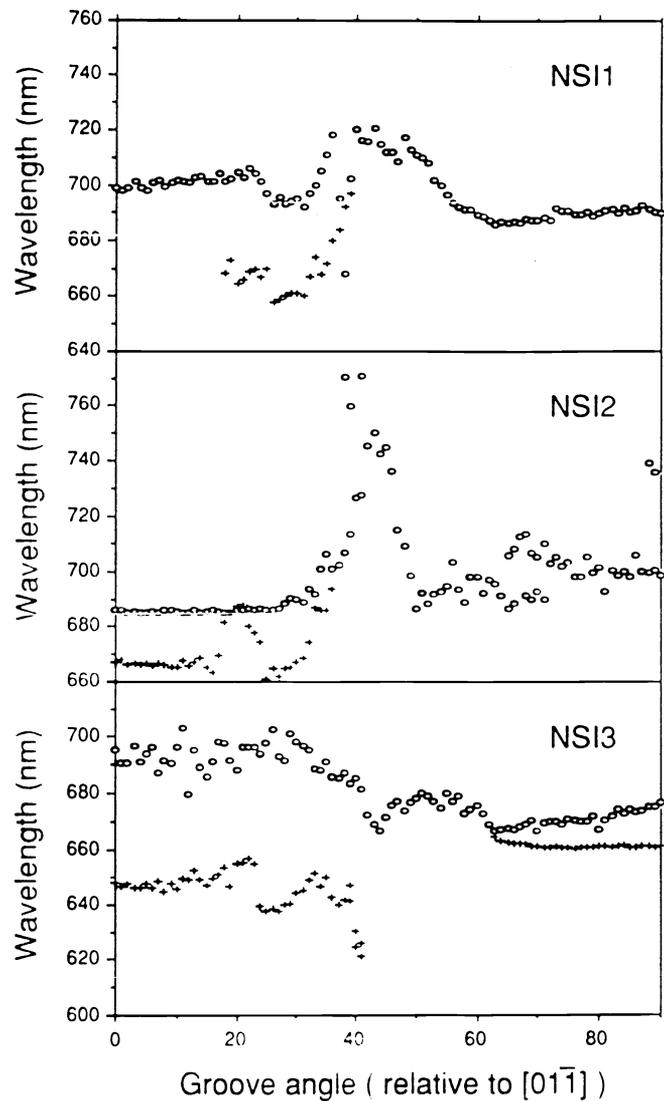
Figure 5: Plot of the AlGaAs peak as a function of groove orientation, relative to the  $[01\bar{1}]$  groove, for NSI1, NSI2, and NSI3. The circles represent luminescence from the side of the grooves, and the '+' symbols represent luminescence from an additional facet at the top of the groove.
