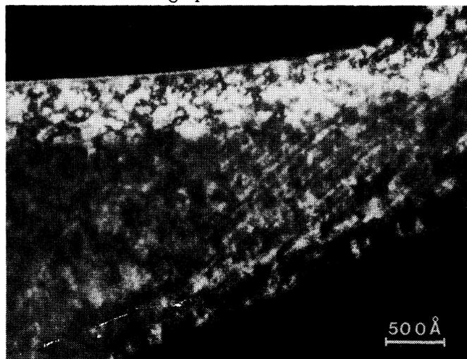
Figure 3: Dark field transmission electron micrograph of a cross section of the groove, showing the interface between the side and bottom facets. The left half of the micrograph shows AlGaAs grown on the bottom of the groove. The right half, in which compositional modulation is seen along the [111] direction, shows AlGaAs grown on the side of the groove. The compositional modulation terminates abruptly at the facet interface.
