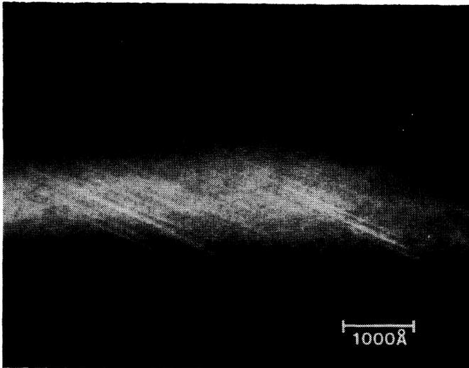
Figure 6: Transmission electron micrograph, taken using the (200)DF condition, of AlGaAs grown on the (211) facet of an  $[01\bar{1}]$  groove, in sample NSI2. Compositional modulation in these layers is observed to intersect the substrate at an angle of  $22^\circ$ . The substrate/epilayer interface contains small (111) facets, approximately  $250\mu\text{m}$  in length, which are associated with an enhancement in the amplitude of the compositional modulation (see text).
