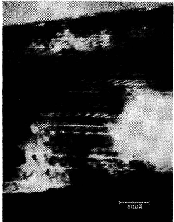
Figure 7: Transmission electron micrograph, taken using the (200)DF condition, of AlGaAs grown on the side of a  $[010]$  groove. Quantum wire-like structures are observed, with a width of approximately  $60\text{ \AA}$ .
