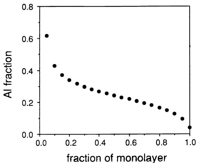
Figure 4: Calculated variation of the composition of columns of atoms added to steps in a (111) facet, with terraces 20 atoms wide, assuming ideal growth by step flow. The growth chamber geometry is described in the text. The aluminum fraction varies by more than 0.5 in the plane of growth.
