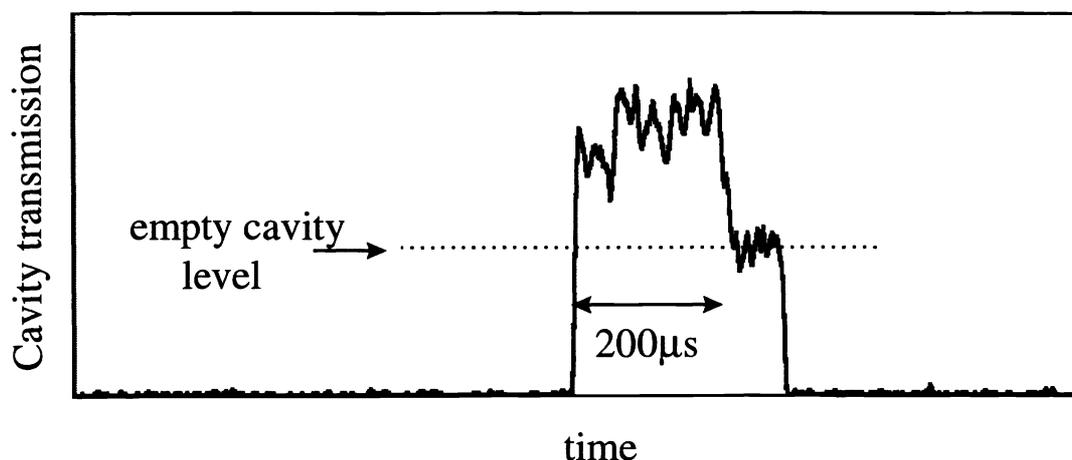
**Figure 4.** Lengthening the interaction time of an atom in the cavity. A probe detuned by  $\simeq -g_0$  is triggered ON in the presence of an atom falling into the cavity mode. Transit times have been extended from  $100\mu\text{s}$  in the absence of forces from this probe field to  $>300\mu\text{s}$ . The transit shown has been extended to  $\sim 200\mu\text{s}$  duration.
