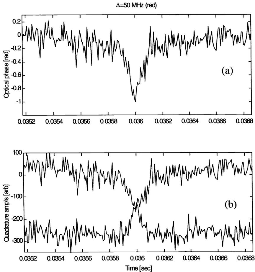
**Figure 5.** Time variation of each quadrature amplitude of the transmitted field (b), and the resulting optical phase (a) for this single atom event.
