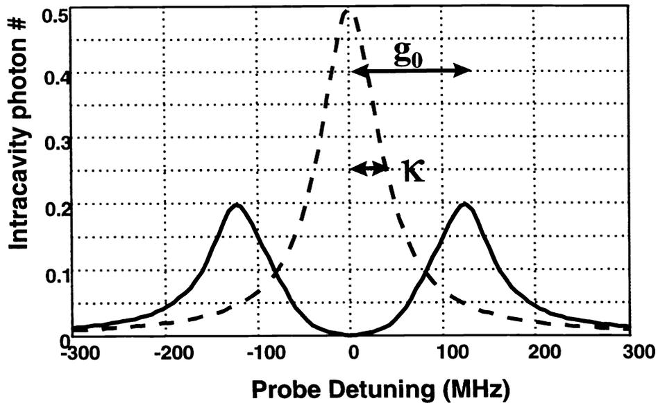
**Figure 2.** Transmission vs. detuning for a probe field of photon number  $=0.5$ , with no atom present (dashed curve), and with a single, optimally coupled atom (solid curve).
