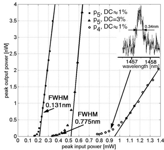
**Figure 10.** Structure  $b_4$ . L-L curve for  $p_5$  and  $p_4$  cavities for two different duty cycles (DC). The pulse periodicity was  $1\mu s$  in both cases. Spectrum taken below threshold, in the case of  $p_4$  cavity is shown in the inset.
