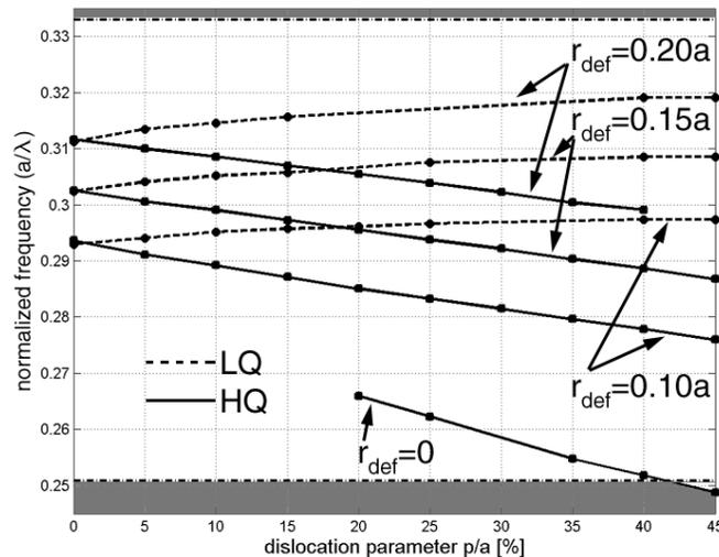
**Figure 3.** Dependence of the position of the two dipole modes of the cavity on the amount of dislocation introduced ( $p$ ), and the size of the defect hole ( $r_{def}$ ).
