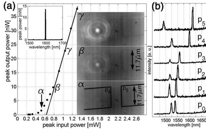
Figure 13. Structure  $a_2 p_4$ . (a) L-L curve. Lasing action occurs from HQ mode positioned at  $\lambda = 1598\text{nm}$ . Insets show spectrum above threshold, and mode profiles of the lasing mode for several pump levels. The boundaries of the structure can also be seen. The mode is very well localized to the center of the cavity. (b) Tuning properties of  $a_2$  structure, as a function of elongation parameter  $p$ .
