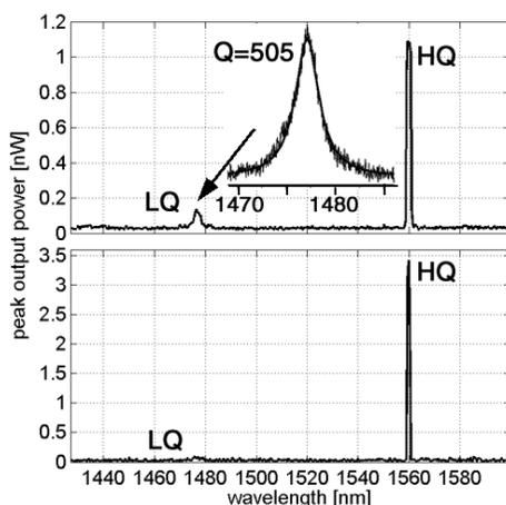
**Figure 11.** Structure  $b_1$ , cavity  $p_5$ . Photoluminescence spectra taken at two different pumping levels. Narrowing of the linewidth in case of HQ mode can be observed. Q-factors of LQ mode are estimated to be around  $Q_{LQ} = 505$ .
