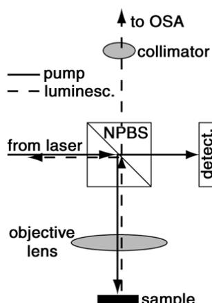
Figure 7. Experimental setup. NPBS stands for Non-polarizing beam splitter.
