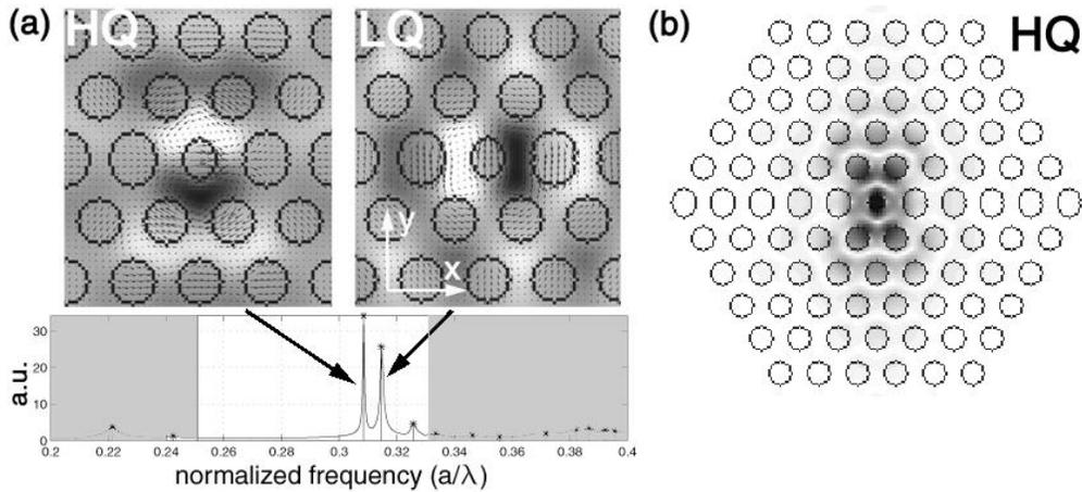
**Figure 2.** Defect modes of the cavity with  $p/a = 10\%$  and  $r_{def} = 0.2a$ . (a) Cavity supports two dipole modes, and their profiles are shown ( $B_z$  component and vector of the  $\vec{E}$  field). Gray shaded region in the spectrum corresponds to the modes of the bulk photonic crystal, while the bandgap is represented with white color. (b) Amplitude of the E field is shown. It can be seen that light is localized in the small defect hole.
