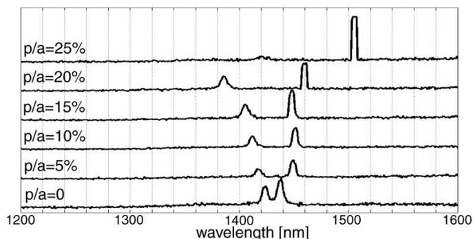
Figure 8. Structure  $b_4$ . Position of resonant modes detected in cavities  $p_0 \div p_5$  as a function of the elongation parameter  $p$ .
