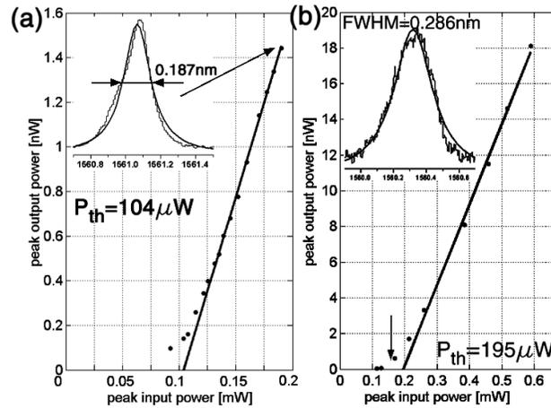
Figure 12. L-L curve of structure  $b_1 p_5$  taken at different pumping levels.  $DC = 1\%$
