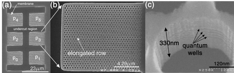
**Figure 5.** SEM micrograph of the structure  $b_4$ . Each structure consists of (a) six different cavities with different elongation parameters:  $p_0 = 0$ ,  $p_1 = 0.05 \cdot a$ ,  $p_2 = 0.1 \cdot a$ ,  $p_3 = 0.15 \cdot a$ ,  $p_4 = 0.2 \cdot a$  and  $p_5 = 0.25 \cdot a$ . (b) Blow-up of  $p_3$  cavity, and (c) of a single hole (tilted). Quantum wells and undercut air region can be seen.
