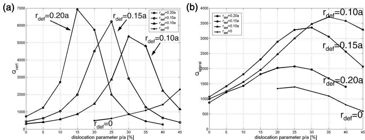
**Figure 4.** Dependence of the (a) vertical and (b) lateral quality factor of the HQ mode on the amount of dislocation ( $p$ ) and the size of the defect hole ( $r_{def}$ ). Only five layers of photonic crystal surrounding the defect hole was used.  $Q_{lateral}$  can be improved by adding more photonic crystal layers.
