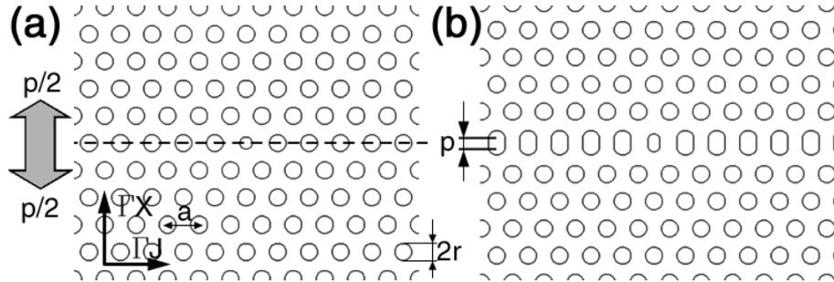
**Figure 1.** (a) Conventional single defect cavity ( $p = 0$ ). When structure is "cut" along the dashed line, and two PPC half-planes are dislocated along  $\Gamma X$  direction by  $p/2$ , (b) high-Q cavity can be formed ( $p = 0.25 \cdot a$ ).
