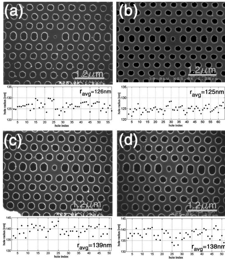
**Figure 6.** SEM micrographs of (a)  $a_2 p_4$ , (b)  $b_1 p_5$ , (c)  $b_4 p_4$  and (d)  $b_4 p_5$  along with the distribution of hole sizes in the bulk photonic crystal mirrors surrounding each cavity.
