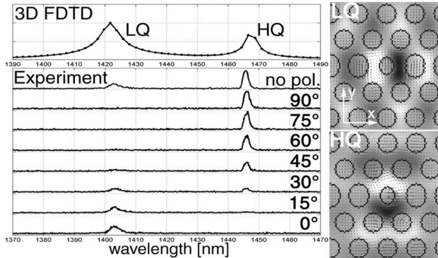
**Figure 9.** Structure  $b_4$ , cavity  $p_3$ . Polarization dependence of the resonant modes.  $0^\circ$  corresponds to y-axis direction. Figure also shows mode profiles ( $B_z$  component), polarization ( $\vec{E}$ ) and position in the spectrum of the LQ and HQ modes, the result of 3D FDTD analysis.
