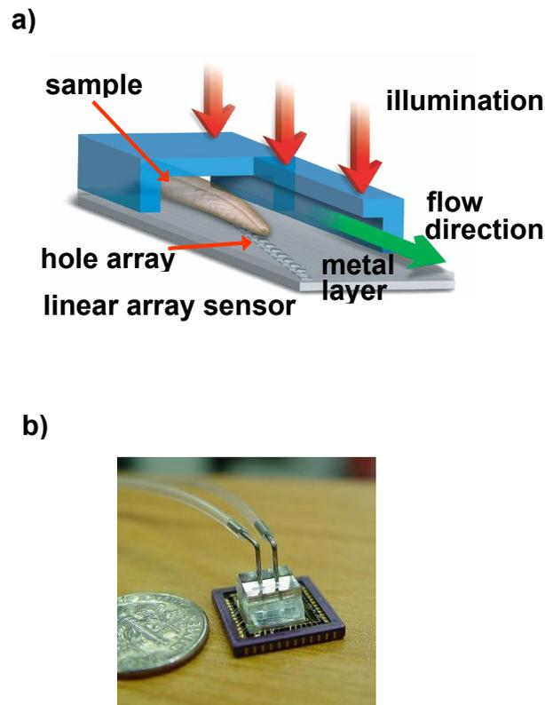
**Figure 2:** **a.** The schematics showing the working principle of the OFM device. **b.** A typical on-chip OFM prototype device, which is about the size of a dime.
