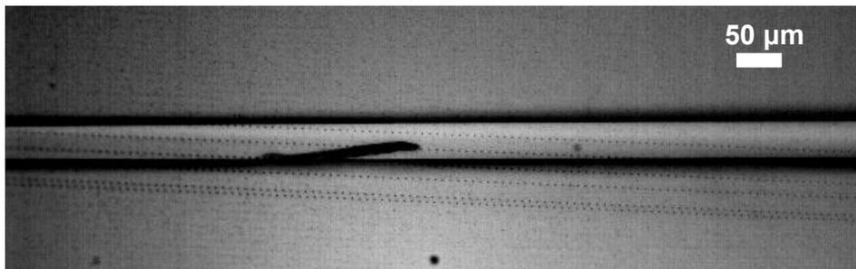
**Figure 4:** **a.** The configuration of two OFM arrays in the prototype device. **b.** A photo showing a *C. elegans* flowing across the two OFM arrays during the OFM imaging experiment.
