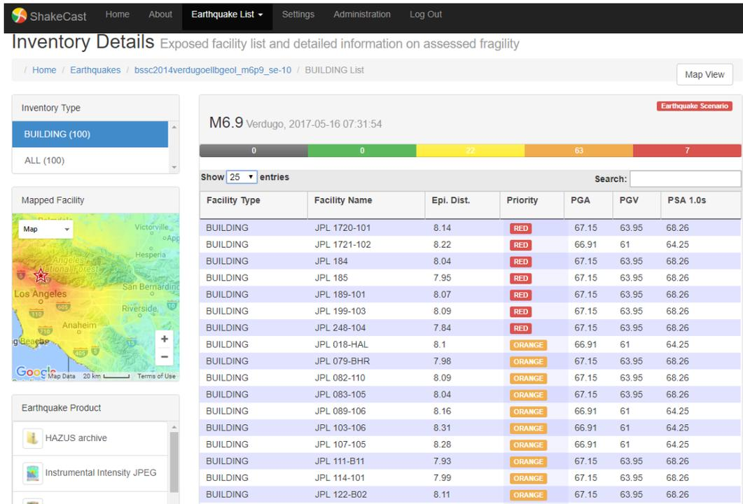
Figure 2. NASA-JPL ShakeCast [5-7] instance showing assessed fragilities in select buildings due to a scenario M6.9 Verdugo fault earthquake near the JPL campus.
