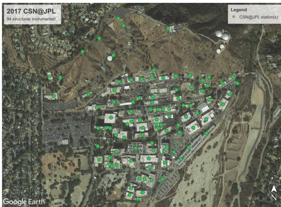
Figure 1. Map of NASA-JPL campus in Pasadena, CA showing locations of CSN accelerometer deployments. Horizontal dimensions are approximately 1 km by 1 km.
