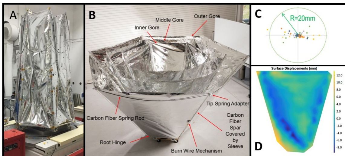
Figure 9. Photon shield deployment demonstration hardware in the JPL Advanced Large Precision Structures (ALPS) Laboratory, and measured flight-like performance results. A: The stowed photon shield system during vibration testing. B: The deployed photon shield met the deployment requirements with significant margin after vibration testing. C: The shield tips deploy to within 4.8 mm rms of the required position, well within the < 40 mm radius requirement. We compiled these measurements over 20 deployments for the 18 tip locations before and after vibration testing. D: Measured surface of an outer gore, giving 2.4^\circ rms large-scale ripple, smoother than the required \pm 15^\circ peak ripple
