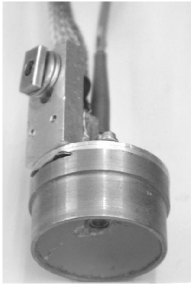
Fig.2. Photo of the resonant photoacoustic transducer.
