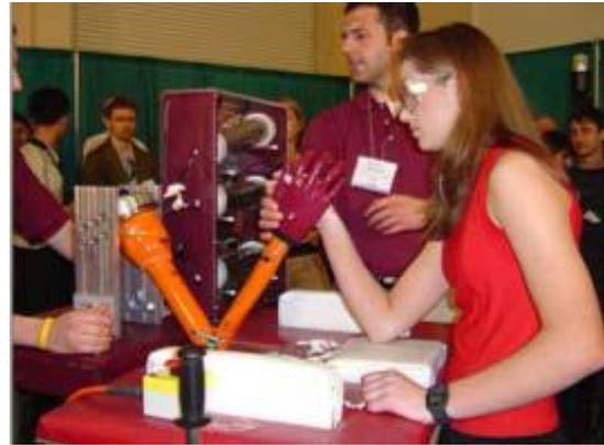
**FIGURE 3:** The fixture that is used to test the force and speed of the EAP actuated robotic arms
