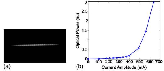
Fig. 6. (Color online) (a) Subthreshold near-field image; (b) a typical optical power versus injection current curve.
