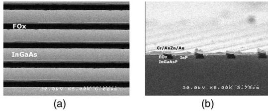
Fig. 4. Scanning electron micrographs of (a) the top view of the F0x overlay that backfilled the trenches and (b) the cross section of a completed device.
