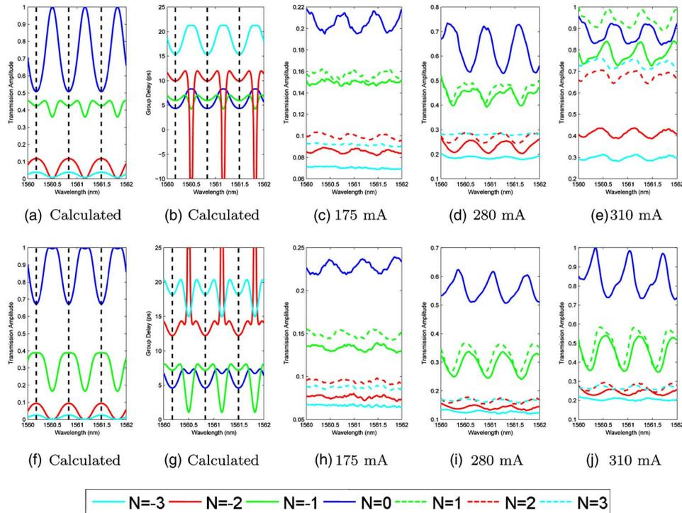
Fig. 8. (Color online) Top row: theoretical (a) transmission and (b) group delay, as well as (c)–(e) experimentally measured transmission spectra at various resonators and injection current amplitudes for an array with an inter-resonator spacing of 800 nm. Bottom row (f)–(j) the same for an array with an inter-resonator spacing of 900 nm.
