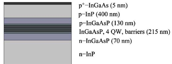
Fig. 2. (Color online) Schematic of the wafer structure.
