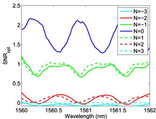
Fig. 9. (Color online)  $\text{SNR}_{\text{opt}}$  as a function of wavelength and resonator position of an array with a transmission spectrum shown in Fig. 8(d).
