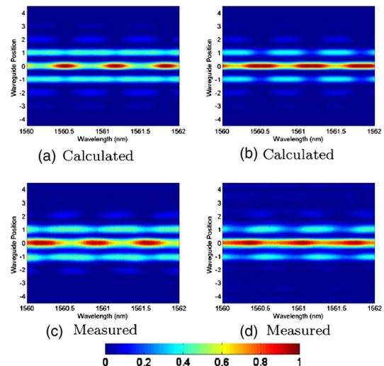
Fig. 7. (Color online) Theoretically calculated transmission spectra for (a)  $\kappa_l=1.1 \times 10^{-3}\ \mu\text{m}^{-1}$  and (b)  $\kappa_l=0.9 \times 10^{-3}\ \mu\text{m}^{-1}$ , and the measured transmission spectra, less the spontaneous emission background, at a current amplitude of 280 mA for an array with inter-resonator spacings of (c) 800 nm and (d) 900 nm.
