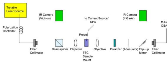
Fig. 5. (Color online) Schematic of the experimental setup. SPA is the semiconductor parameter analyzer and OSA is the optical spectrum analyzer.
