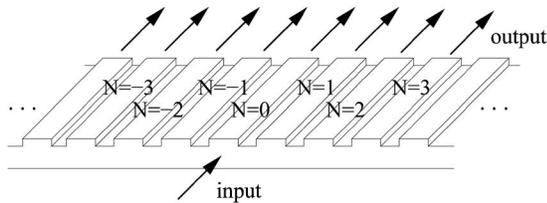
Fig. 1. Schematic of the Fabry-Perot resonator array CROW.
