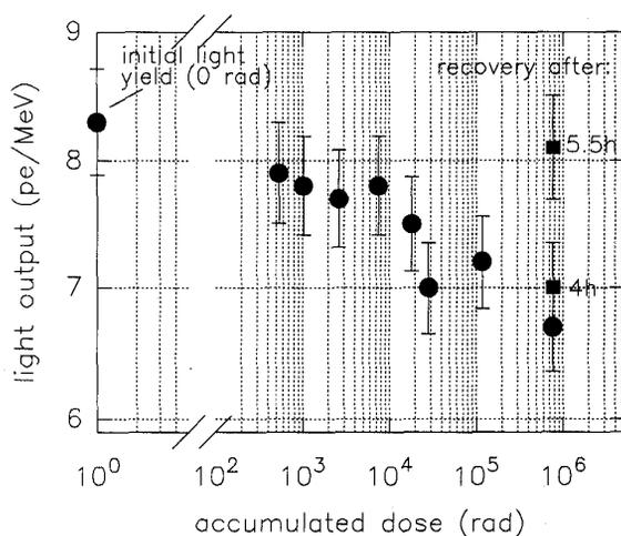
**Figure 4:** Light output vs accumulated dose for sample 767. Except where indicated, all points were measured approximately 30 minutes after irradiation.
