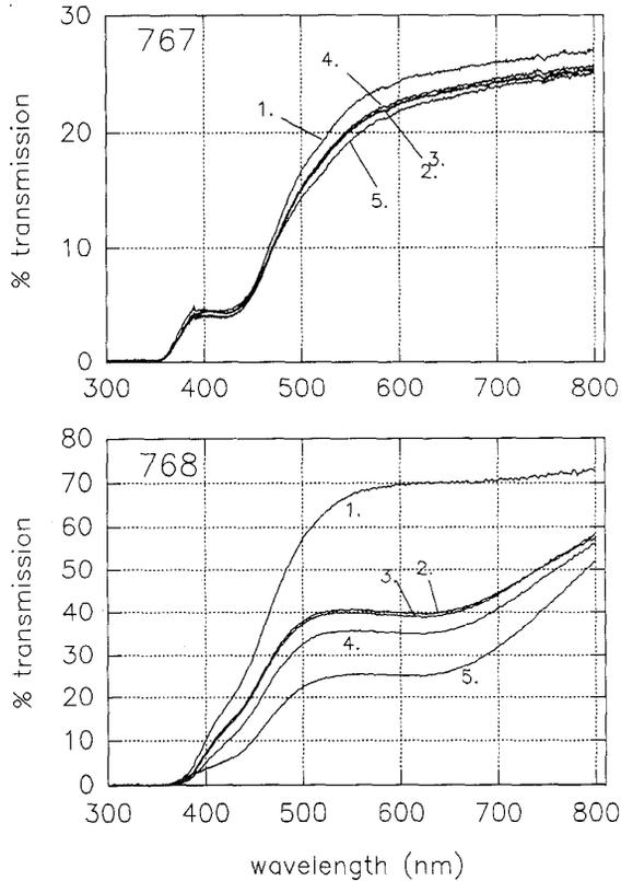
**Figure 1:** Longitudinal transmission spectra as a function of radiation dose for samples 767 and 768. Cumulative doses for 767 are 1 - initial, 2 - 2.6 Krad, 3 - 7.6 Krad, 4 - 18.2 Krad, 5 - 769 Krad. Dose rate was 120 rad/hr for doses 2 through 4 and  $3.5 \times 10^4$  rad/hr for dose 5. Cumulative doses for 768 are 1 - initial, 2 - 2.4 Krad, 3 - 11 Krad, 4 - 20 Krad, 5 - 834 Krad. Dose rate for dose 2 through 4 was 132 rad/hr and  $3.6 \times 10^4$  for dose 5.
