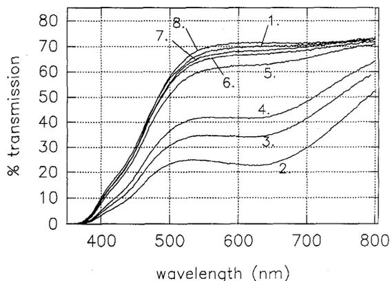
**Figure 6:** Effect of optical bleaching on sample 768. Longitudinal transmission curves correspond to: 1- initial; 2- immediately after a total dose of 834 krad; optical bleaching: 3- 5 hours at 700 nm; 4- 12 hours at 700 nm; 5- 5 hours at 600 nm; 6- 10 hours at 600 nm; 7- 7 hours at 640 nm; 8- 2 hours of thermal annealing at 200°C.
