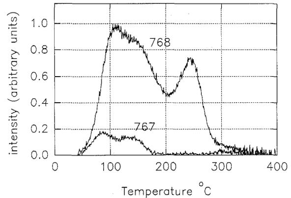
**Figure 8:** Thermoluminescence glow curves for samples 767 and 768.
