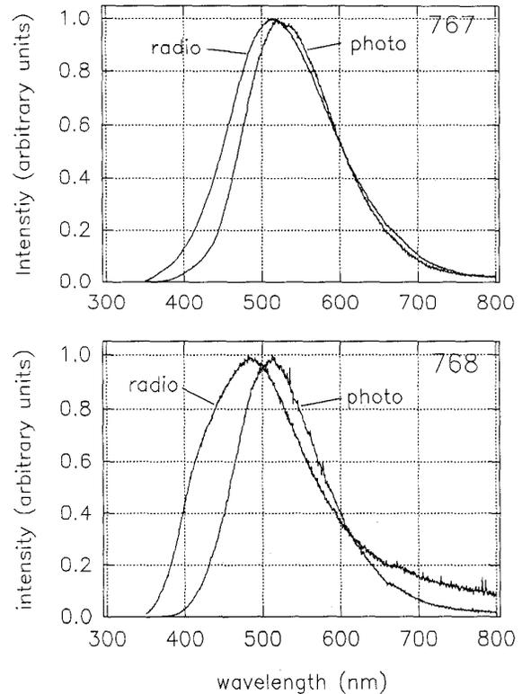
**Figure 2:** Radioluminescence and photoluminescence emission spectra for samples 767 and 768. All spectra have been corrected for phototube quantum efficiency and monochromator efficiency and normalized to one at their peak.
