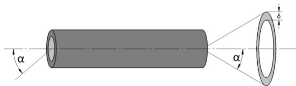
Figure 3- Condition observed in a fiber fed with a beam having no divergence, i.e. the input beam has NA=0 . Incorrect aiming with respect to the optical axis of the fiber results in a ring of light at the input angle.
