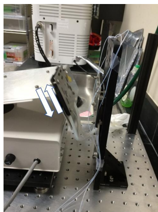
Figure 10. Dynamic bending scrambler
