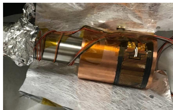
Figure 8. Left top: Flexible copper thermal strap. Right top: Kapton heater. Left bottom: One of the pulse-tube cryocooler. Right bottom: Temperature control unit for the coldhead
