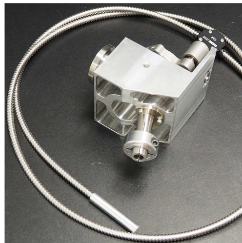
Figure 5. Left: cross section of the fiber port used by the first version of the FIU plate. Right: picture of the fiber port with the dummy bundle used during the mechanical tests.
