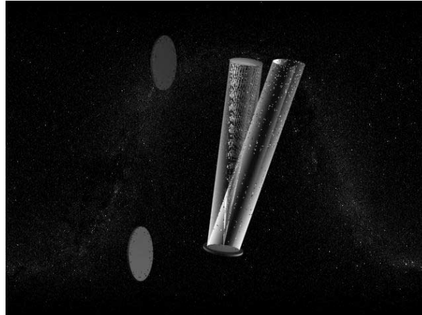
Figure 1: Spacecraft formation flying geometry for ASSiST. Starlight entering from the top-right is collected by a Schmidt corrector mirror (bottom) then focused by the F/10 primary mirror (top). Also shown are two large sunshades (at left), which may be inflatable. The instrument bus resides behind the corrector mirror.
