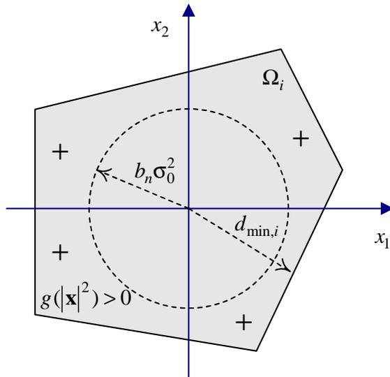
Fig. 5. Two-dimensional illustration of the problem geometry for the case  $d_{\min,i}^2 \geq b_n \sigma_0^2$ . The decision region  $\Omega_i$  is shaded.  $g(|\mathbf{x}|^2)$  has a sign as indicated by “+” and “-”.
