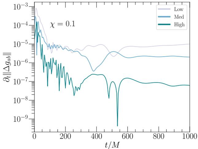
FIG. 5. Behavior of the derivative of the norm of the metric perturbation with time for a background with spin  $\chi = 0.1$ . We plot  $\partial_t \|\Delta g_{ab}\|$ , the time derivative of the norm of the metric perturbation. Each line corresponds to a different resolution. We see that after an initial period of junk radiation, the time derivative is convergent towards zero with increasing numerical resolution.
