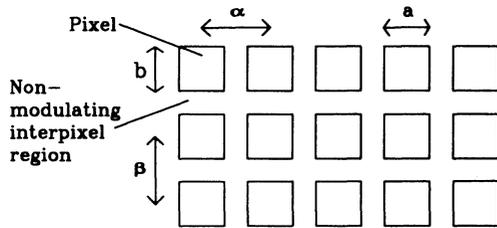
Fig. 3 Model of the LCTV screen.
