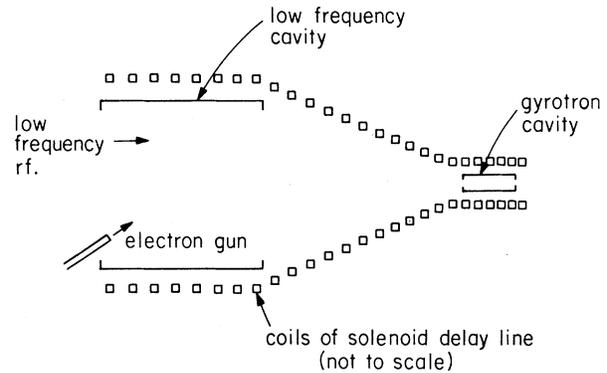
FIG. 4. Proposed pulsed gyrotron.
