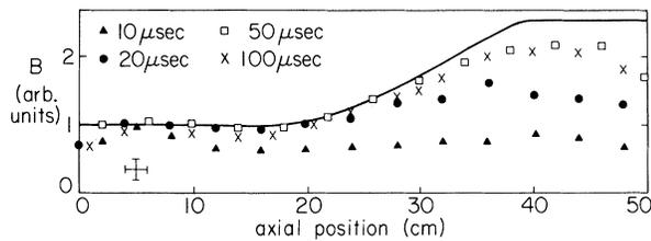
FIG. 3. Observed  $B$  dependence on position compared with Eq. (5) (solid line) for four different pulse durations. Bars at lower left show typical error.
