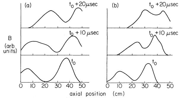
FIG. 2. Observed propagating compressing mirrors, input pulse: (a) 20  $\mu$ sec max, 20  $\mu$ sec min, 20  $\mu$ sec max (equal amplitude maxima); (b) 5  $\mu$ sec max, 17  $\mu$ sec min, 9  $\mu$ sec max (first maximum has 40% more amplitude than second).
