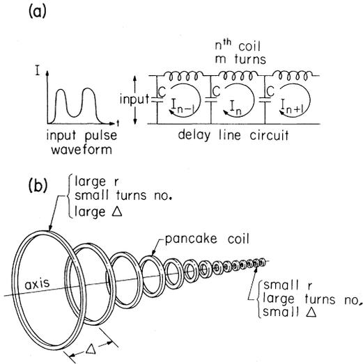
FIG. 1. (a) Circuit and input pulse; (b) physical configuration.  $\Delta$  is the intercoil spacing. For the device described here coils 1-7 have  $r=4$  cm,  $m=10$ ,  $\Delta=3$  cm; coils 8-15 are the tapered section; coils 16-24 have  $r=2$  cm,  $m=19$ ,  $\Delta=2$  cm.
