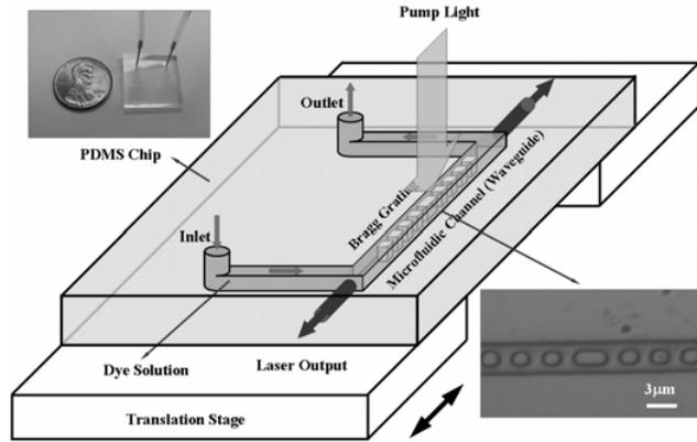
Fig. 1. Schematic diagram of a tunable optofluidic DFB dye laser chip. The upper inset shows an actual PDMS laser chip. The translation stage movement stretches or compresses the PDMS chip along the Bragg grating direction. The resulting grating period change causes the lasing wavelength to shift. The lower inset is an optical micrograph of the central phase-shifted region of the laser cavity. The grating period is 3080nm and total length is 1cm. The channel is 2μm high and 3μm wide.
