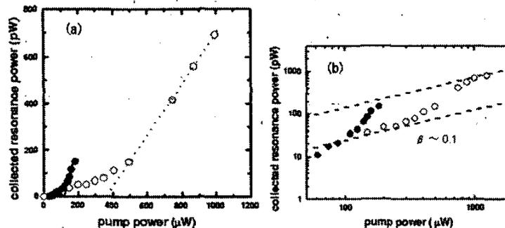
Fig. 1. Collected resonance power as a function of peak pump power. Panels (a) and (b) show the linear-linear plot and the log-log plot. Filled circles and open circles are data from two-defect coupled cavity and four-defect coupled cavity.
