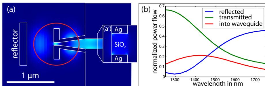
Fig. 1. (a) Optimized optical Yagi-style antenna. Field distribution  $|E_y|$  in the substrate plane, obtained from a full 3D FDTD simulation. Simulating the excitation with a Gaussian beam of N.A. 0.9 from air (red circle). (a') Field distribution in a cross section with  $300\text{ nm} \times 300\text{ nm}$  gap size. (b) Reflection, transmission and coupling efficiency of an antenna, which is optimized for  $\lambda = 1550\text{ nm}$ .
