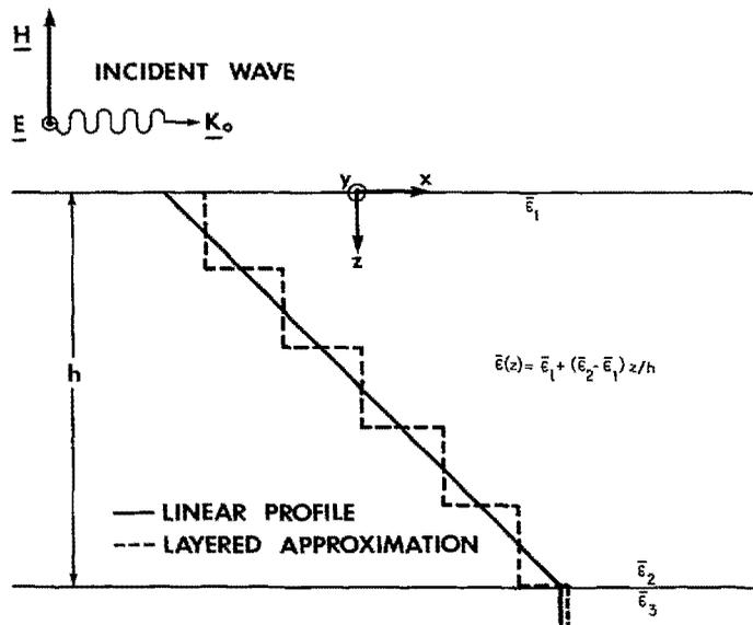
Fig. 1. Dielectric profiles. Complex dielectric constant  $\bar{\epsilon}(z)$  varies linearly from value  $\bar{\epsilon}_1$  at surface to  $\bar{\epsilon}_2$  at homogeneous half-space. In examples under consideration,  $\bar{\epsilon}_2 = \bar{\epsilon}_3$ , which is value in homogeneous half-space.
