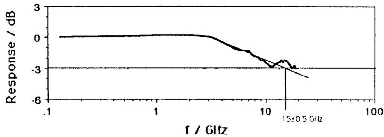
Figure 3. Frequency performance of the 'hybrid' waveguide detector used in the WDM array.
