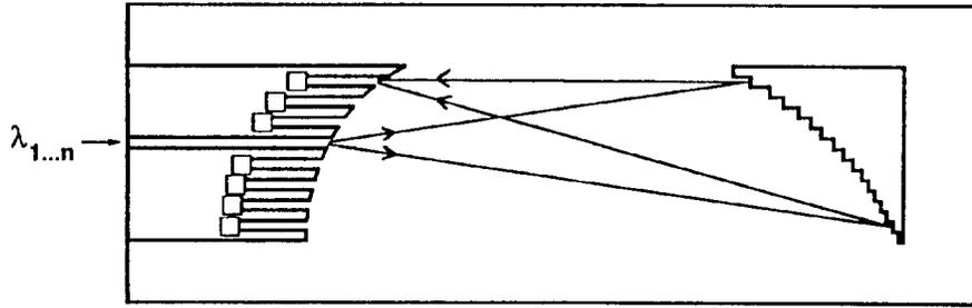
Figure 1. Schematic of the monolithic WDM detector chip.
