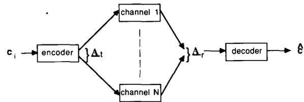
Fig. 3. Communications channel model of feature measurement.
