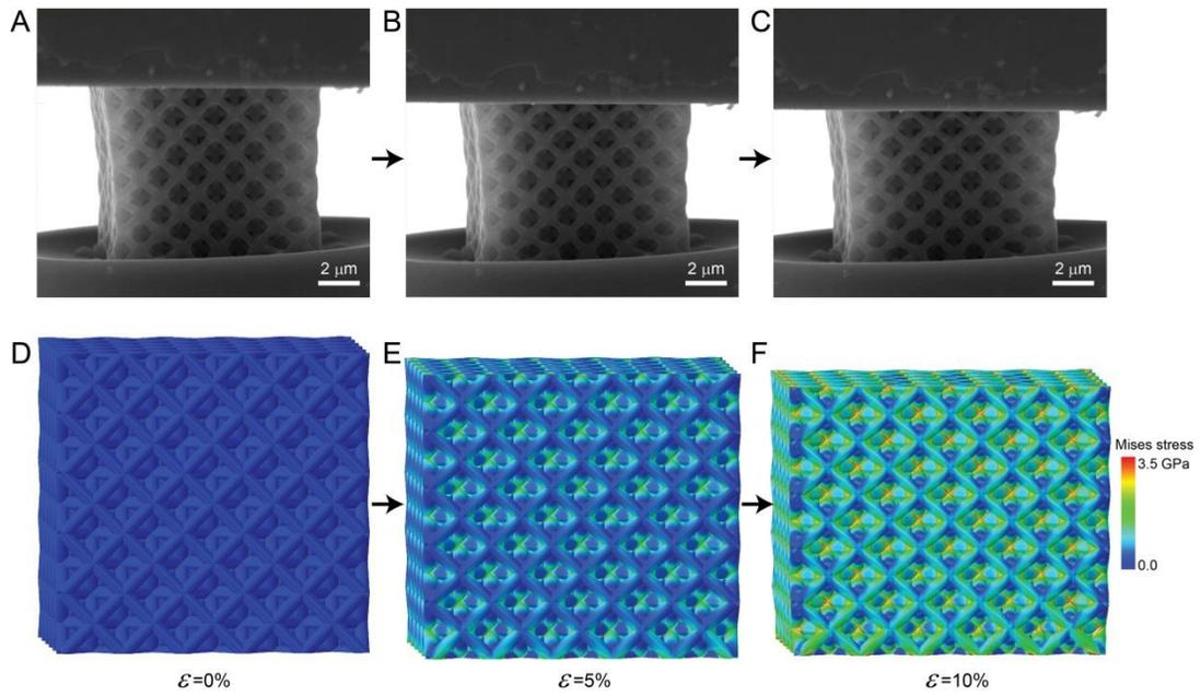
**Fig. S6.** Comparisons of deformation snapshots in octet-truss nanolattice with relative density of 37.5% from finite element modelling and in-situ experiments. (A, B, C) SEM images from in-situ testing at different strains. (D, E, F) Snapshots from finite element modelling with solid elements at different strains.
