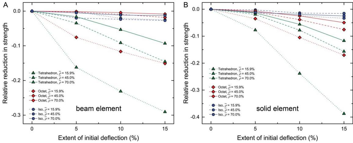
**Fig. S5.** Relative reduction in strength of nanolattices as a function of the extent of initial deflection. (A, B) Results from finite element modelling based on beam and solid elements.
