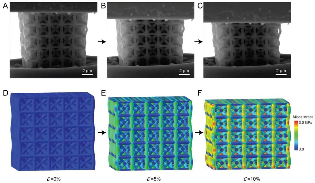
**Fig. S7.** Comparison of deformation snapshots in an iso-truss nanolattice with relative density of 39.4% from finite element modelling and in-situ experiments. (*A, B, C*) SEM images from in-situ testing at different strains. (*D, E, F*) Snapshots from finite element modelling with solid elements at different strains.
