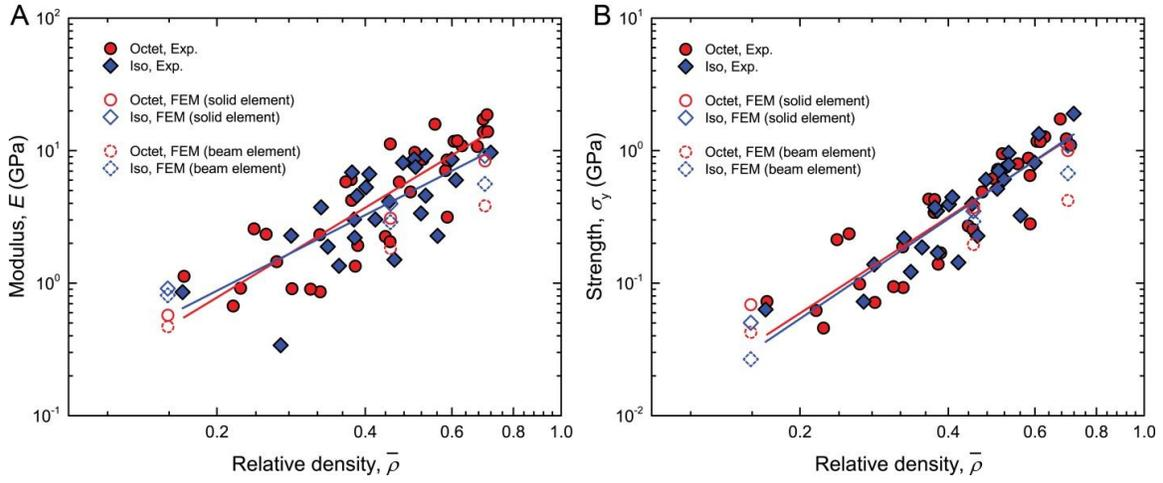
**Fig. S4.** Comparison between finite element modelling and experimental results. (A, B) Modulus versus relative density and strength versus relative density from finite-element modelling and experiment. While the modelling results based on solid elements are in good agreement with those from experimental measurements, those based on beam elements exhibit similar trend but larger deviations from experiments at higher relative densities.
