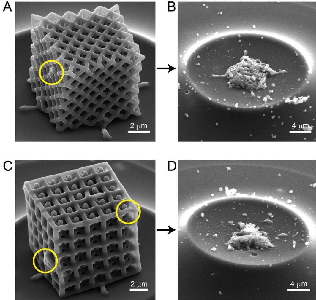
**Fig. S1.** SEM images of typical octet- and iso-truss nanolattices before and after compression. (A, B) SEM images of an octet-truss nanolattice with  $d=382$  nm. (C, D) SEM images of the iso-truss nanolattice with  $d_1=538$  nm and  $d_2=612$  nm. The images in (B) and (D) indicate brittle failure of nanolattices.
