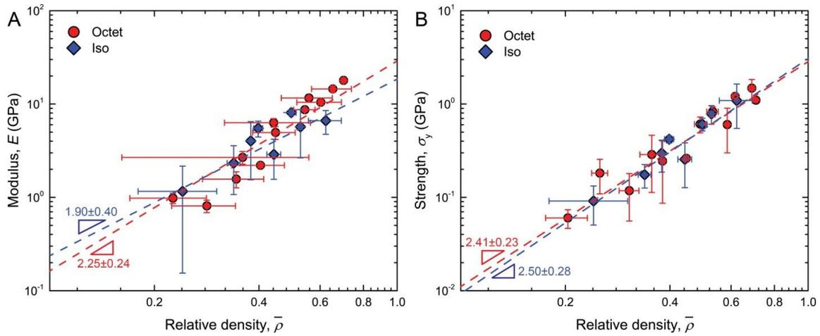
**Fig. S3.** Young's modulus and compressive strength versus density of pyrolytic carbon nanolattices. (A,B) Young's modulus and strength versus relative density of octet- and iso-truss pyrolytic carbon nanolattices on log-log scale. Scaling power law slopes are indicated for each architecture. Error bars represent the standard deviations from the average over some data of samples with comparable densities.
