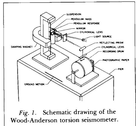
Fig. 1. Schematic drawing of the Wood-Anderson torsion seismometer.
