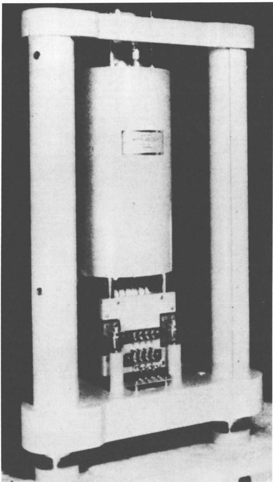
Fig. 2. Hugo Benioff's vertical component seismometer.
