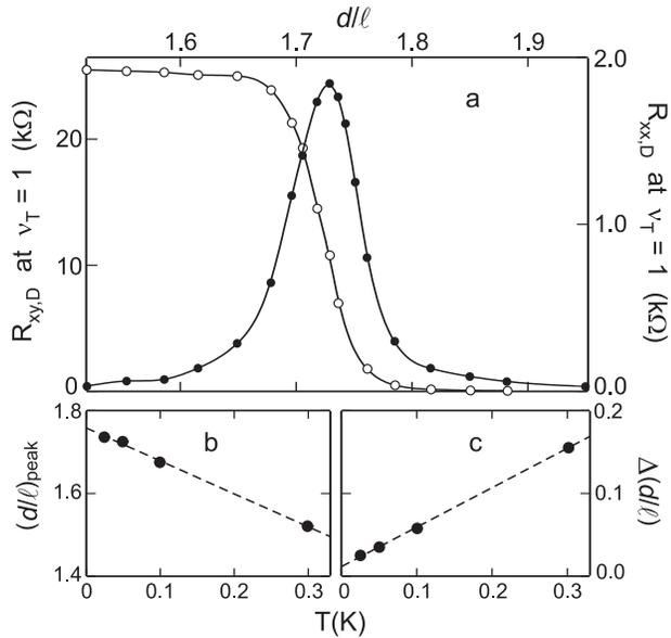
FIG. 2: a) Hall (open dots) and longitudinal (closed dots) drag at  $\nu_T = 1$  and  $T = 50\text{mK}$  vs.  $d/\ell$  in sample B. b) and c) Temperature dependence of location and half-width of peak in  $R_{xx,D}$  at  $\nu_T = 1$ . Lines are guides to the eye.
