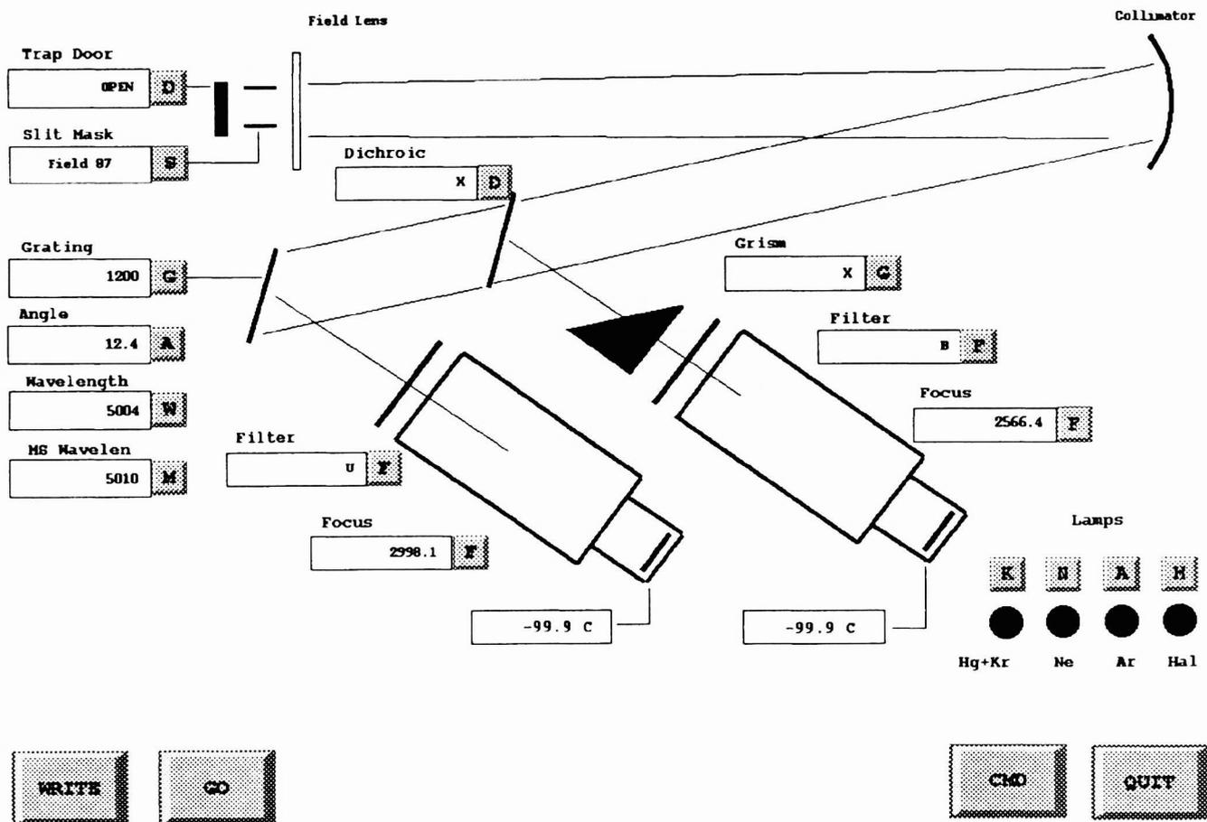
**Figure 5.** The XLRIS graphical user interface for control of all instrument functions, both blue and red. The small grey buttons activate pop-up menus with which the astronomer may select from among the available optics, set camera focus, or set the tilt of the red grating. The large grey buttons along the bottom are used to create or invoke setup "scripts" which initiate numerous configuration changes in parallel.
