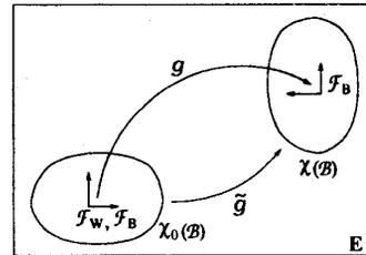
Fig. 7. A configuration specified as  $\mathcal{F}_B$ 's location relative to  $\mathcal{F}_W$ .
