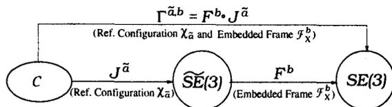
Fig. 3. C-space representation diagram.
