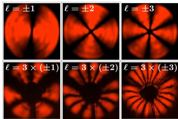
FIG. 3. **Coherent OAM multiplication.** Top row: Near field of input coherent superpositions. Bottom row: Tripled output states. The number of petals is  $6|\ell|$ , as expected from a coherent operation.
