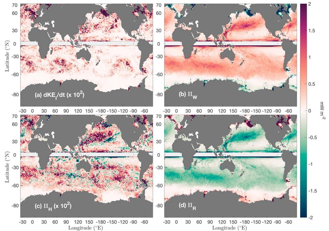
**Figure 11.** Annual-mean estimates of (a) rate of change in  $KE_I$ , (b)  $\Pi_W$ , (c)  $\Pi_H$ , and (d)  $\Pi_R$  (in  $\text{mW/m}^2$ ) calculated from LLC 1/48° hourly wind stress and ocean currents. Note the change in scale: (a) and (c) are two orders of magnitude smaller than (b) and (d).
