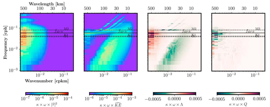
**Figure B1.** Frequency-wavenumber spectrum for wind stress (first panel), kinetic energy (second panel), cospectrum of wind stress and ocean surface currents (third panel), and quadrature spectrum of wind stress and ocean surface currents (fourth panel).
