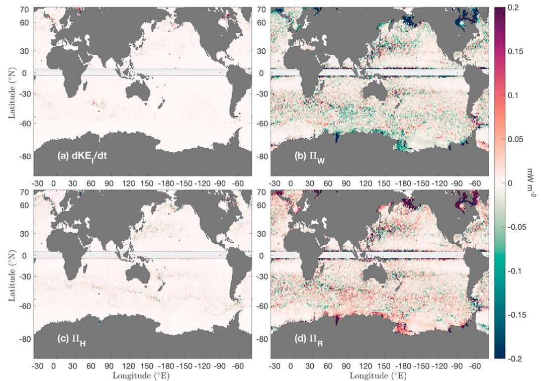
**Figure 12.** Annual mean of the difference between LLC 1/48° and LLC 1/24° estimates of near-inertial kinetic energy budget terms. (a) Rate of change in  $KE_I$ , (b)  $\Pi_W$ , (c)  $\Pi_H$ , and (d)  $\Pi_R$  (in  $mW/m^2$ ) calculated from hourly wind stress and ocean currents.
