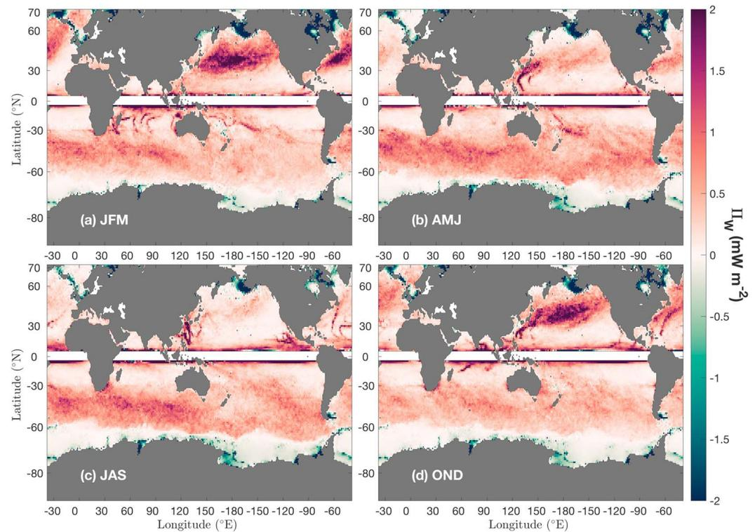
**Figure 6.** Seasonal (3-month averaged for (a) JFM, (b) AMJ, (c) JAS, and (d) OND months) maps of surface kinetic energy flux at near-inertial band ( $\Pi_w$ , in  $\text{mW/m}^2$ ) calculated from hourly wind stress and ocean currents, both filtered at the near-inertial band.
