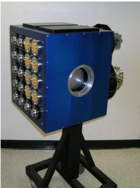
Figure 8: The SuperCam cryostat
