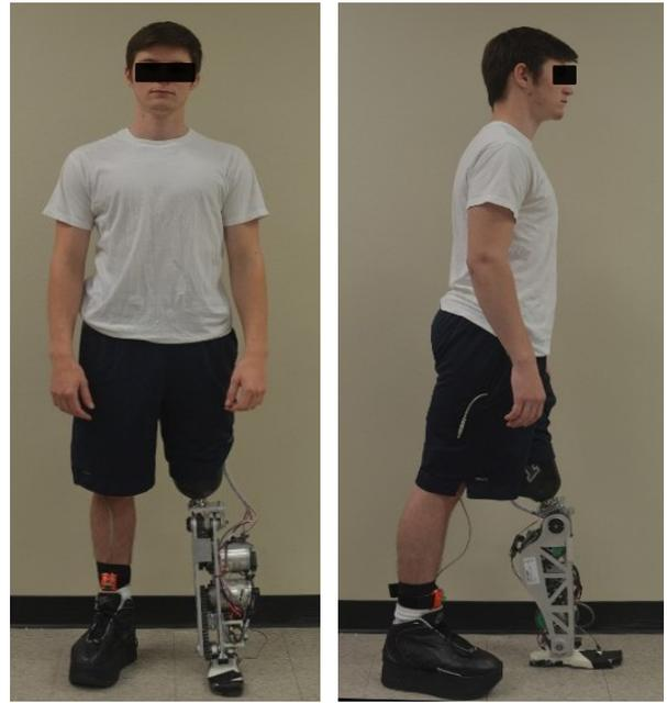
Fig. 1: Transfemoral test subject wearing the custom built prosthetic device, AMPRO.
