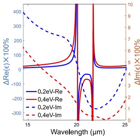
**Fig. 4.** Relative change of the effective in-plane dielectric permittivity,  $\epsilon_0$ , of the metamaterial, for two different Fermi levels, namely  $E_F = 0.2$  eV (blue curves) and  $E_F = 0.4$  eV (red curves), with respect to the case  $E_F = 0$  eV. Solid curves (left y-axis) correspond to real parts and dashed curves correspond to imaginary parts (right y-axis).
