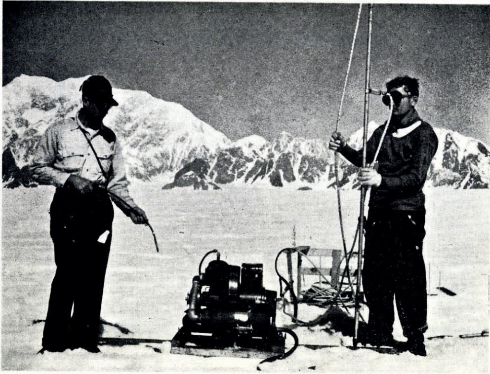
Fig. 2. Thermal boring equipment. Man at left holding thermohm (see text, p. 479)
