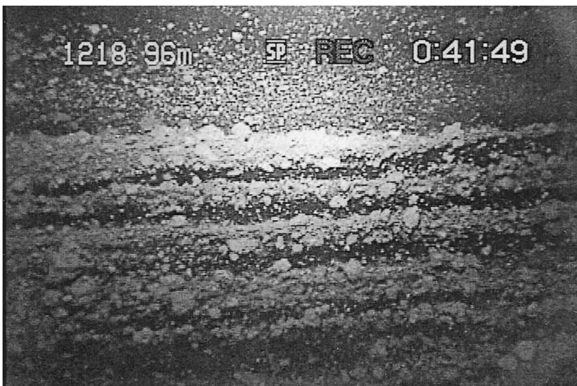
Fig. 7. Debris strata. Accretion of basal ice in the presence of saturated sediments could generate ice lenses of this type. Each image covers about 4 cm in the vertical at the ice wall. These strata are a few millimeters in thickness and separation. Note the clarity of the ice in the lenses. (Up in the figure is down in the ice.)
