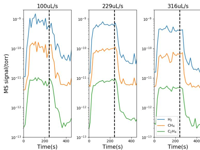
Figure S1. Effect of electrolyte flow rate. Chronoamperometry (CA) was carried out over a copper foil for 240 (s) at different flow rates. The black dashed line indicates where the CA ends.
