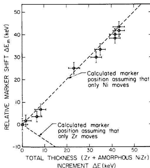
FIG. 2. Amount of displacement of the W marker,  $\Delta E_m$ , vs the amount of displacement of the Ni-amorphous NiZr interface,  $\Delta E$ . Both quantities are measured relative to those of the sample annealed for 30 min at 300 °C (see Fig. 1). The two dashed lines correspond to the energy shift of the W marker under the assumption that either Ni or Zr is the only diffusing species.
