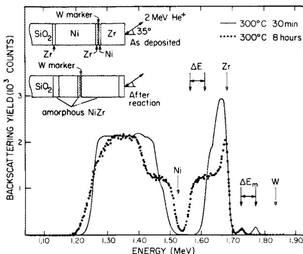
FIG. 1. 2.0 MeV  $35^\circ \text{He}^+$  backscattering spectra of a Ni-W (4 Å)-Zr sample (insert) annealed for 30 min and 8 h at 300 °C. The displacement of the marker peak position and of the Ni-amorphous NiZr interface half-height position, are shown by  $\Delta E_m$  and  $\Delta E$ , respectively. The spectra were taken with 1.66 keV/channel.
