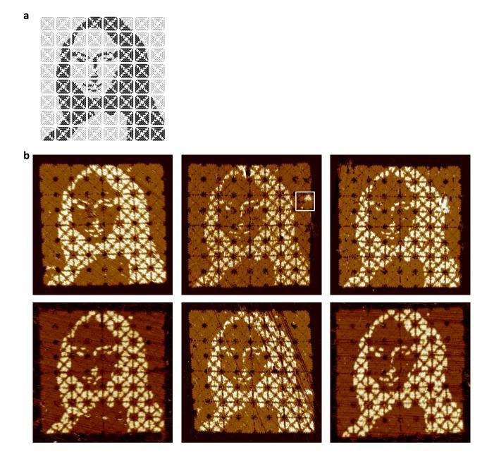
Figure 17: 8 by 8 arrays with a pattern of Mona Lisa. a, Design diagram. b, AFM images. Tiles with an incorrect pattern are highlighted with a white square frame. The correct tile incorporation rate was estimated as  $99.79 \pm 0.09\%$ , averaged over thirty eight images including the six shown here.
