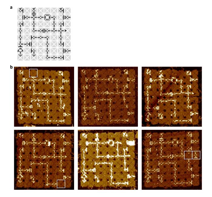
Figure 20: 8 by 8 arrays with a pattern of a photoreceptor circuit.<sup>31</sup> a, Design diagram. b, AFM images. Tiles with an incorrect pattern are highlighted with a white square frame. The correct tile incorporation rate was estimated as  $98.96 \pm 0.52\%$ , averaged over the six images.
