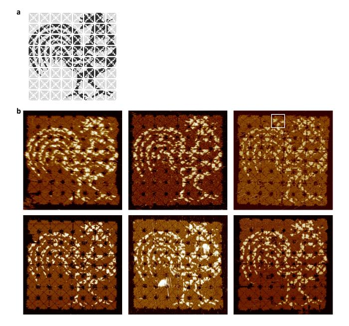
Figure 18: 8 by 8 arrays with a pattern of a rooster. a, Design diagram. b, AFM images. Tiles with an incorrect pattern are highlighted with a white square frame. The correct tile incorporation rate was estimated as  $99.74 \pm 0.26\%$ , averaged over the six images.
