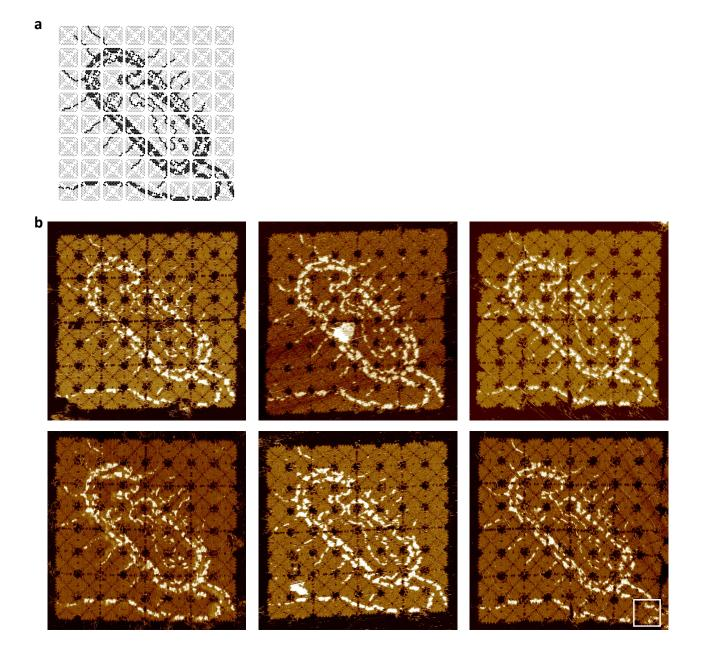
Figure 19: 8 by 8 arrays with a pattern of a bacterium. a, Design diagram. b, AFM images. Tiles with an incorrect pattern are highlighted with a white square frame. The correct tile incorporation rate was estimated as  $99.74 \pm 0.26\%$ , averaged over the six images.
