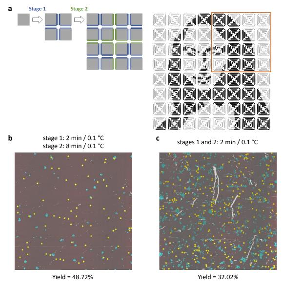
Figure 16: Annealing time. a, Design diagram of a quadrant of the 8 by 8 fractal assembly with an example pattern of Mona Lisa. AFM image of the quadrant annealed for b, 2 min per 0.1 °C in the first stage and 8 min per 0.1 °C in the second stage, and c, 2 min per 0.1 °C in both stages.
