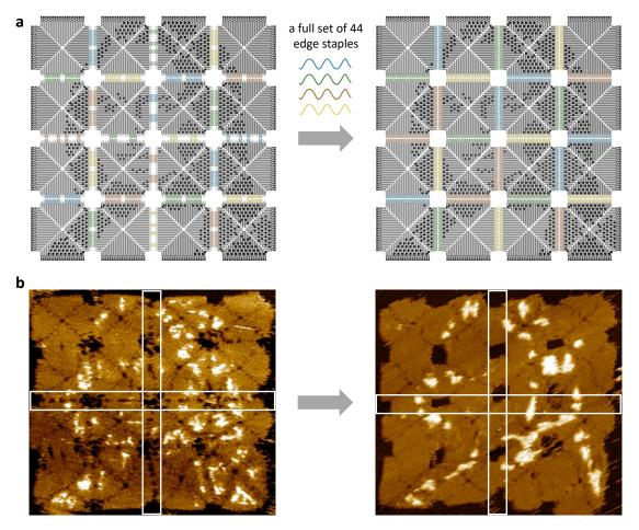
Figure 22: Strengthening the origami arrays after fractal assembly. a, Design diagram of a 4 by 4 array strengthened by adding a full set of 44 edge staples with stacking bonds after the fractal assembly. b, AFM images of the 4 by 4 array before and after strengthening. The white boxes highlight the most obvious changes in the number of edge staples.
