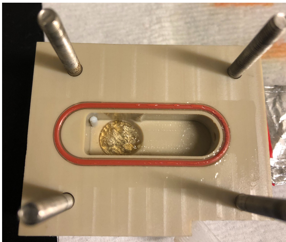
Figure S22. Picture of the cell and cathode after electrocarboxylation with a magnesium anode
