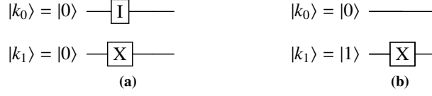
Figure 1: A basic quantum circuit with two qubits k_0 and k_1 . As indicated in (b) the identity gate I is usually omitted in circuit diagrams so that circuits (a) and (b) are equivalent. The states of both qubits are initialised with |k_0\rangle = |0\rangle and |k_1\rangle = |0\rangle so that |q\rangle = |k_0\rangle \otimes |k_1\rangle = |0\rangle \otimes |0\rangle which is abbreviated as |q\rangle = |00\rangle . The output of the circuit is (I \otimes X)(|0\rangle \otimes |0\rangle) = I|0\rangle \otimes X|0\rangle = |0\rangle \otimes |1\rangle .
