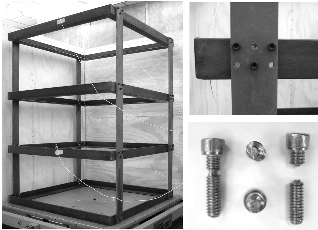
Fig. 1. Instrumented steel frame (left), close-up of bolted beam-column connection (top right), and notched bolts before and after failure (bottom right). Dimensions are shown in Fig. 2.
